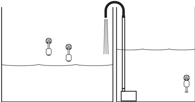
The pump will continue to run until ONE of the primary OR secondary float switches are submerged.
