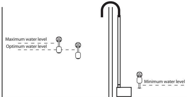
1. Find the point in the sump where the water level will fluctuate. This is usually the section that contains the return pump.
