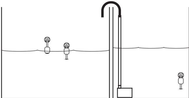
However, if the water level of the reservoir drops below the reservoir float switch, the pump will stop to prevent the pump from running dry and causing damage to the pump.
