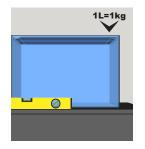
Place the aquarium on a level surface strong enough to support the weight of the aquarium, all equipment, substrate, ornaments and water in the aquarium. Note that water is heavy (1kg per litre).
