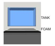
Always place the sheet of foam provided between the aquarium and the surface to absorb any irregularities. Failure to do so may result in damage to the aquarium.
